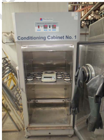
Figure 6: Photo of equipment to measure the mass flux in the steady-state regime.
