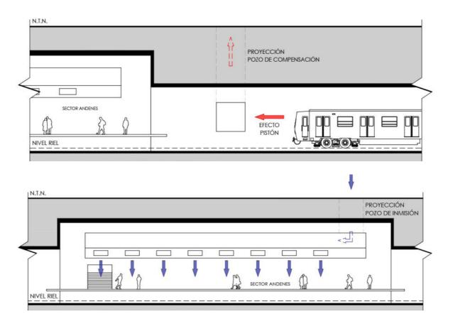
Figura 4. Longitudinal view of compensation wells. Source: Made by the author based on Herrero (2009). Figura 5. Longitudinal view of immission wells. Source: Made by the autorbased on Herrero (2009).
