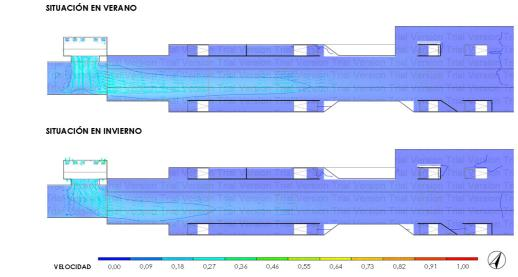
Figura 15. Air speed for the existing situation. Source: Made by the author.
