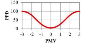
Figura 10. Thermal sensation scale according to Fanger method. Source: Made by the author based on Arballo Kuchen, Alamino-Naranjo and Alonso-Frank (2016).
