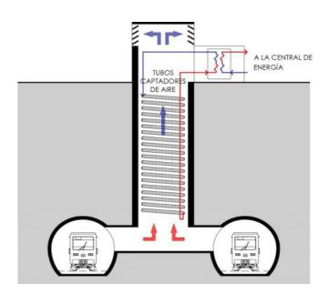
Figura 9. Operation of the heating system in the Northern Line. Source: Made by the author based on Arden (2013).
