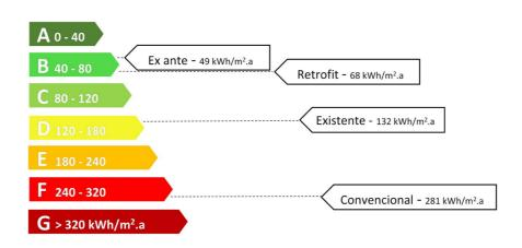
Figure 6. Energy Efficiency Label as per IRAM 11900:v.2017. IPE Values.Source: Preparation by the authors
