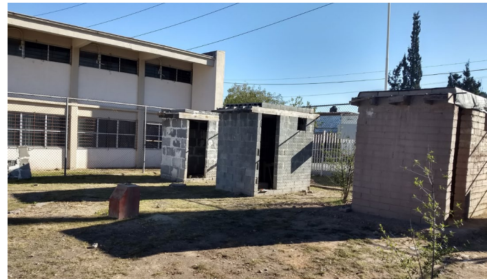
Figure 2. View of the modules (from left to right: egg carton blocks with Thermolite and cement – ECB, concrete block – CB, and compressed earth block – CEB). Source: Preparation by the author.
