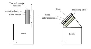
Figure 1. Solar chimney setups. Source: Harris & Helwig (2007, p. 136).
