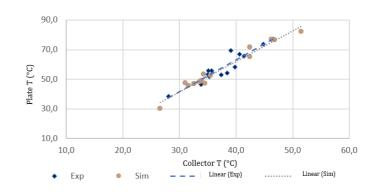
Figure 5. Correlation between air temperature and plate temperature.
