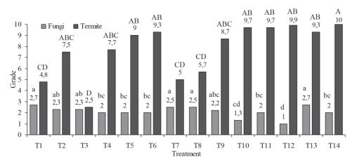
Figure 2. Average deterioration rates, assigned on the basis of the analysis of the occurrence and action of fungi and termites in wood thermorectified *Eucalyptus grandis*, exposed in the test field after ten months.
