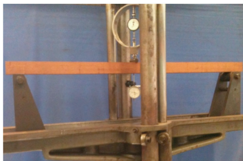
Figure 1. Bending test in Hymenaea stilbocarpa wood specimen.
