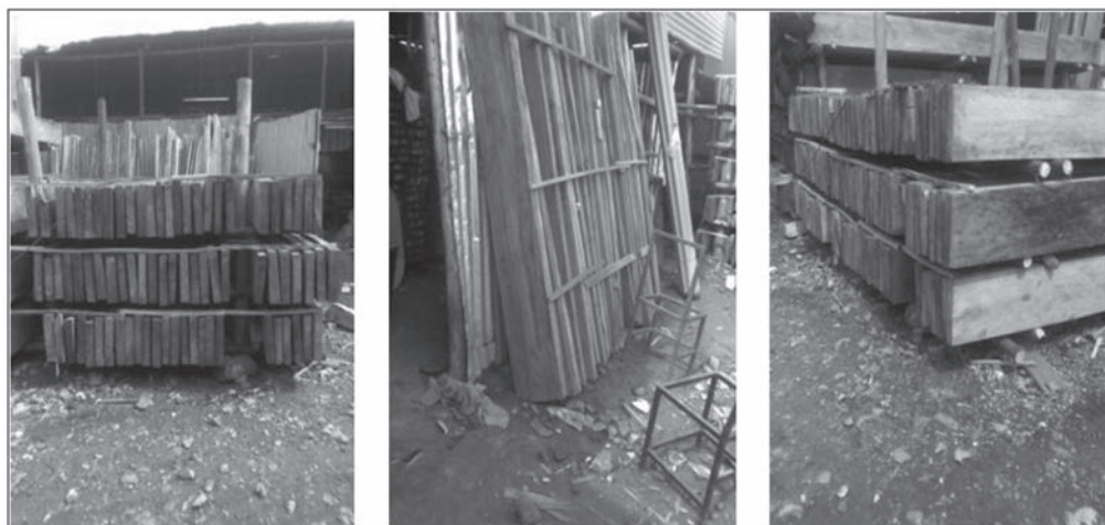
Figure 1. Improper timber stacks in carpentry workshops at Bwaise, Kampala District.
