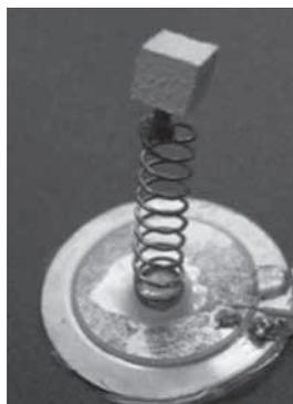
**Figure 2.** Earlywood specimen mounted on piezoelectric sensor.
