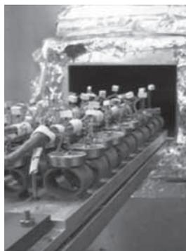
**Figure 3.** Specimens on the Dynamic Sorption platform
