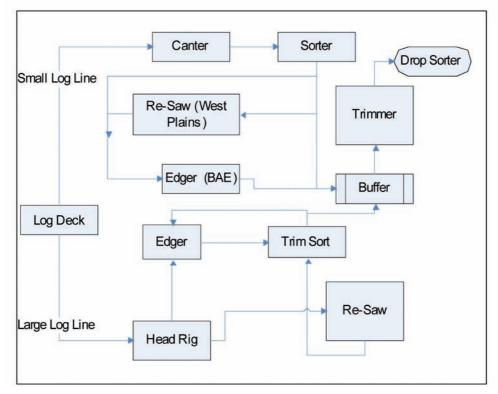
Figure 1: Sawmill layout and flow
