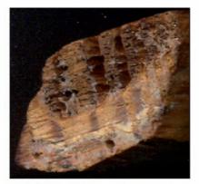
**Figure 4.** Details of degradation by *Gloeophyllum sepiarium* on non-impregnated pinewood  $(T_0)$ .
