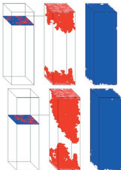
Figure 3: Drying in a 30x30x98 three-dimensional cubic network
