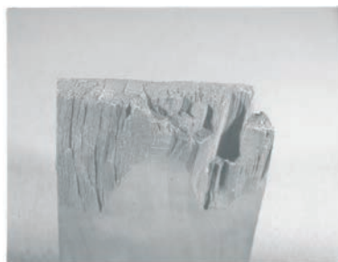
Fig. 3a The typical fracture of a completely treated Poplar specimen after a bending test
