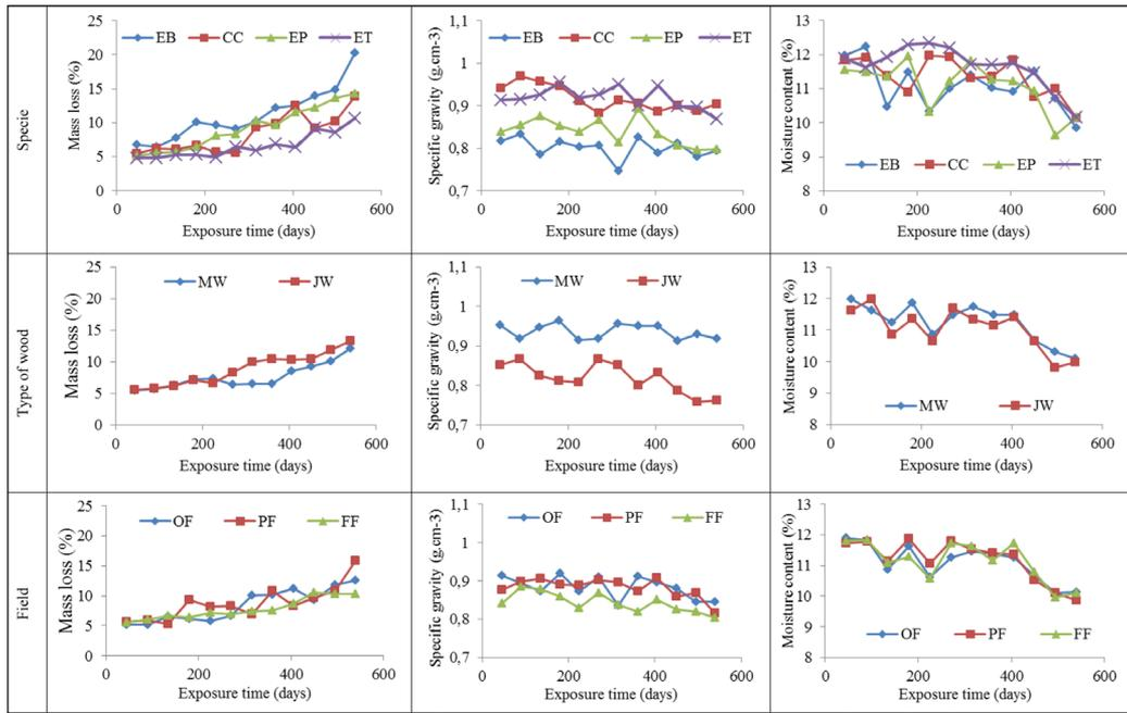
**Figure 2.** Variation of mass loss, density and moisture content against exposure time to the field test.
