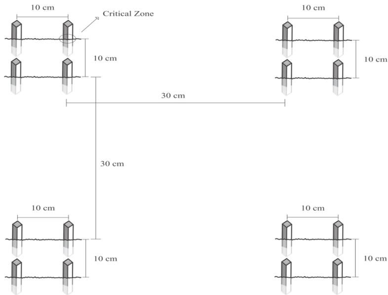
**Figure 1.** Schematic of the samples in the field tests.
