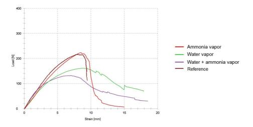
Figure 4. Load-displacement curves of mean values for treated and untreated samples.
