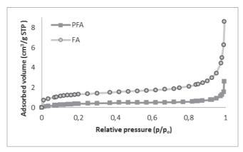
Figure 6. N, adsorption isotherm at -196 °C for FA and PFA.
