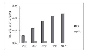
**Figure 8.** CO, adsorption capacity of FA and PFA at different temperatures.
