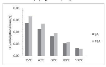
**Figure 7.** CO<sub>2</sub> adsorption capacity of BA and PBA at different temperatures.
