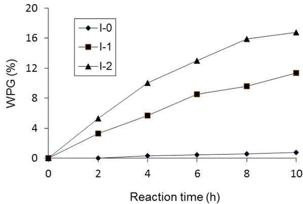
**Figure 2.** Plot of WPG versus reaction time for IPA modified rubber wood at 95°C. Catalyst (iodine) concentrations are: I-0 = 0 mol L<sup>-1</sup>; I-1 = 0,02 mol L<sup>-1</sup>; and I-2 = 0,035 mol L<sup>-1</sup>.
