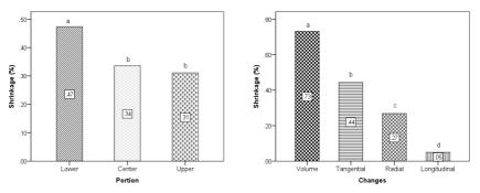
**Figure 5.** Shrinkage properties of juvenile *N. cadamba* wood at different portions (left) and wood changes according to volumetric and dimensional (right).
