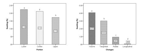
Figure 6. Swelling properties of juvenile *N. cadamba* wood at different portions (left) and wood changes according to volumetric and dimensional (right).
