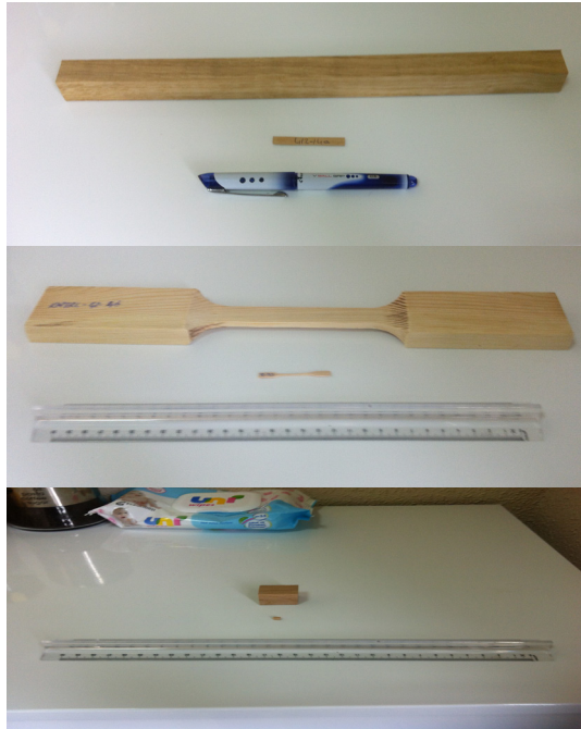
Figure 4. The micro- and standard-size test samples for bending (upper) tension (middle), and compression (bottom).
