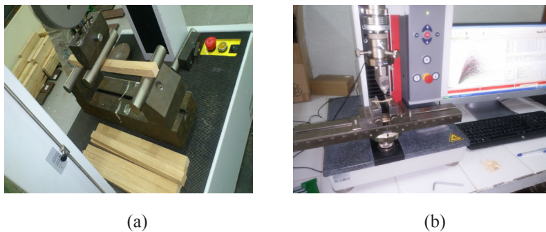
Figure 2. Standard-size bending test sample and test setup (a) and micro-size bending test sample and test setup (b).
