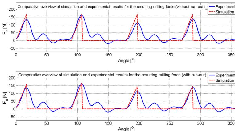
Figure 5. Comparative overview of simulation and experimental results for the resulting milling force  $F_R$ .
