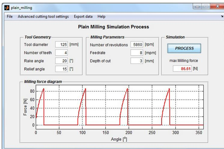
Figure 4. Representation of the application for the milling process simulation.
