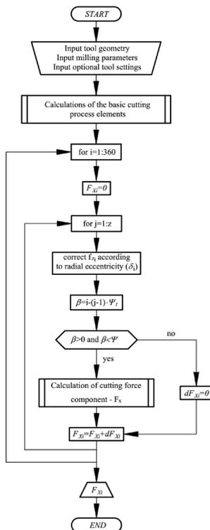
**Figure 1.** Flowchart for determining current values of the milling force components ( $F_{xi}$  - current value of the milling force,  $f_{zi}$  - feed per tooth,  $\delta_i$  - tooth radial run-out/ radial eccentricity  $dF_x$  - current elementary value of the milling force component,  $\psi_t$  - cutter pitch angle,  $\psi$  - engagement angle,  $\beta$  - current engagement angle).
