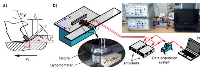
**Figure 2.** a) Scheme of forces in peripheral up - milling ( $v_F$ -feed rate,  $c_D$ -cutting depth,  $f_z$ -feed per tooth,  $a$ -current milling thickness,  $\psi$ - engagement angle,  $F_x$  and  $F_y$ -components of milling forces), b) Scheme of equipment setup for experimental determination of forces in peripheral milling.
