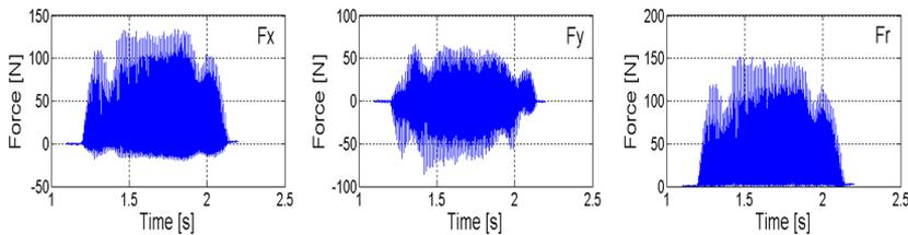
**Figure 3.** Diagrams of the milling forces records.
