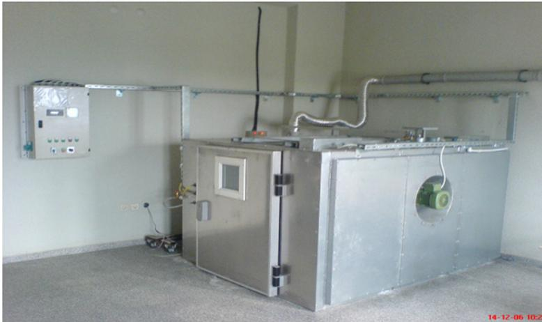
Figure 1. Drying kiln used for the trials.
