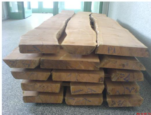
**Figure 6.** Lumbers dried with the non-protective drying schedule.
