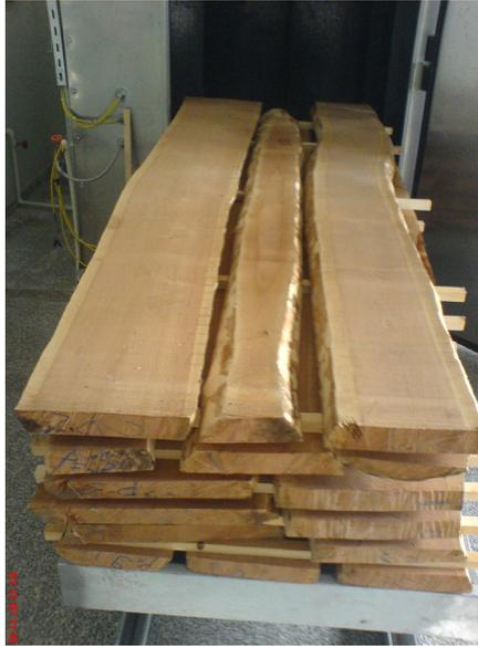
**Figure 7.** Lumbers dried with the protective drying schedule.
