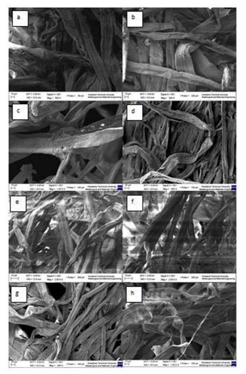
Figure 1. SEM photographs of the enzyme eucalypts and pine kraft pulp: (a) control of pine kraft pulp; (b) XyzGeo71 treatment of pine kraft pulp; (c) LipRHA1 treatment of pine kraft pulp; (d) consecutive XyzGeo71 and LiPRHA1 treatment of pine kraft pulp; (e) control of eucalypts kraft pulp; (f) XyzGeo71 treatment of eucalypts kraft pulp; (g) LipRHA1 treatment of eucalypts kraft pulp; (h) consecutive XyzGeo71 and LiPRHA1 treatment of eucalypts kraft pulp; (h)
