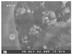
**Figure 1.** SEM images of paper-sheets filled with PCC: (a) unmodified precipitated calcium carbonate; (b) modified precipitated calcium carbonate under conditions of 4% CMC, 0.8% PAC and pH of 7,5 (magnification 2000x).
