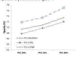
**Figure 7.** The effect of different addition levels of PCC modified with 4% CMC 0,8% PAC in pH=7,5 on opacity.
