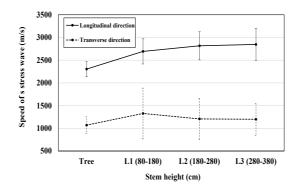
Figure 3: Stress wave velocity in trees and logs of Paulownia wood.
