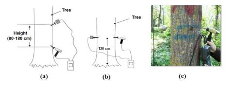
Figure 1: Schematic of tree measurement using stress wave NDT (a) longitudinal direction, (b) transverse direction and (c) real photo.
