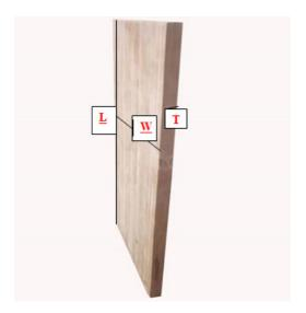
Figure 1: The three planes of the laminated bamboo.
