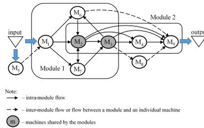
**Figure 5:** Network representation of a baseline facility layout under study with related material flow.
