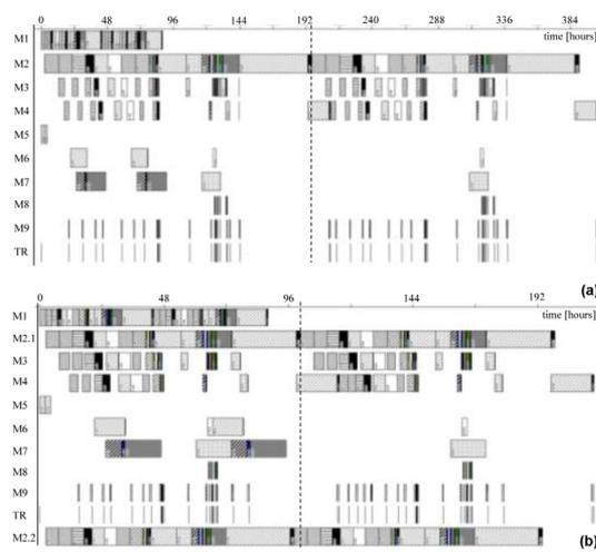
**Figure 6:** Gantt chart of operational schedule solution for the baseline system layout (scenario), i.e. with single machine  $M_2$ , disclosed as a bottleneck (a) and for process layout with duplicated machine  $M_2$  (b); the bold dashed lines show the end of the first repetition and the start of the second repetition of the  $M_2$  (a bottleneck machine) production cycle, each one associated with the realisation of all assigned process operations for complete product spectrum.
