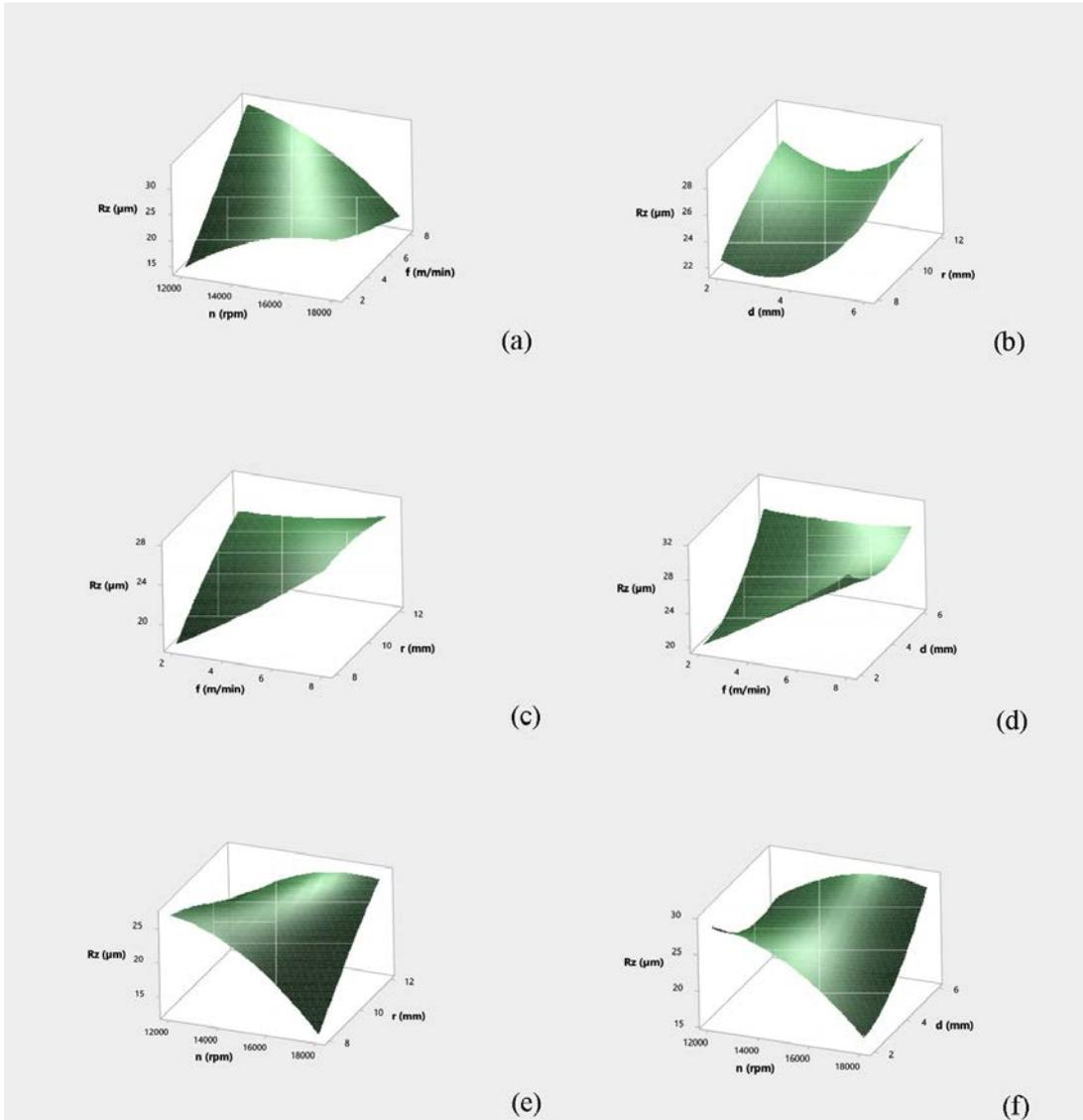
Figure 6: According to 3D surface plots (a, b, c, d, e, f) of different values processing parameters for  $R_z$ .
