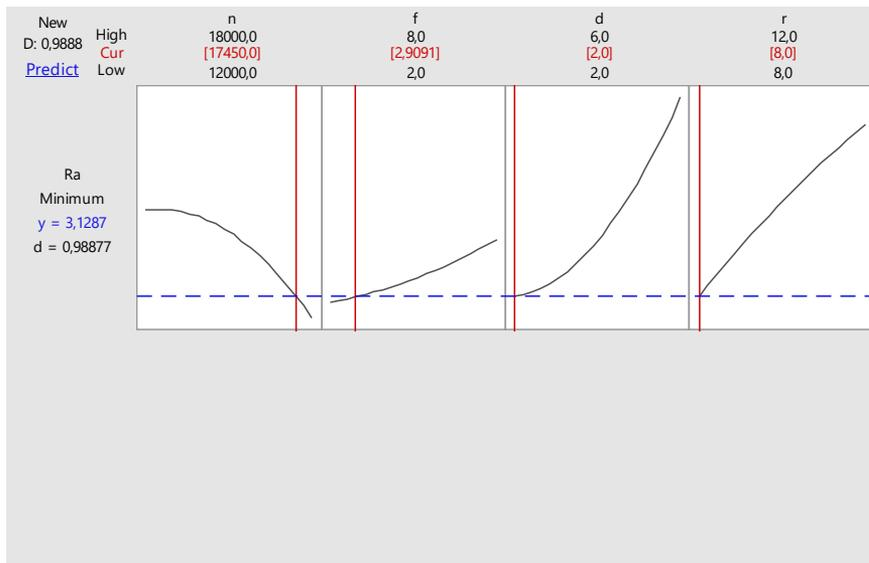
**Figure 7:** Response optimization plot for  $R_a$ .
