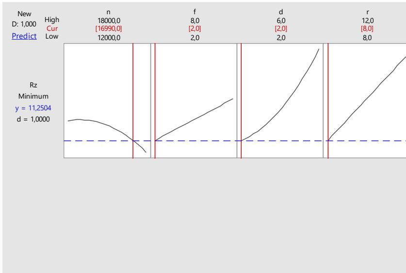
Figure 8: Response optimization plot for  $R_z$ .
