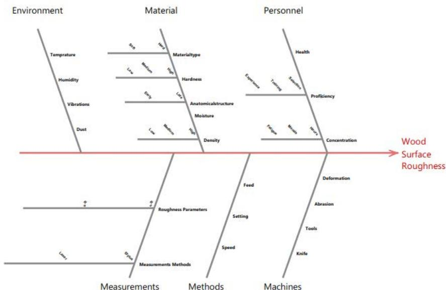
Figure 1: Cause and effect diagram of wood surface roughness parameters.
