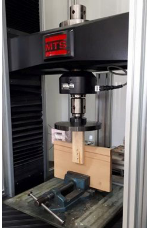
Figure 4: Test set-up for evaluating lateral shear load resistance of staple-connected wood joints.
