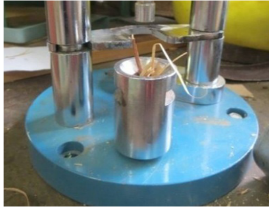
Figure 3: Handle device for pelletization (10 mm diameter and 12-14 mm length).
