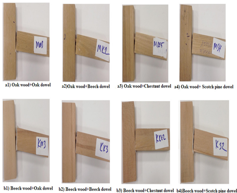
Figure 4: Mode of T-type, two pins dowel joint failure not reinforced.
