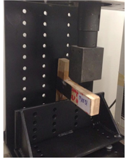
Figure 3: Way of support and loading the specimens of the corner joints.
