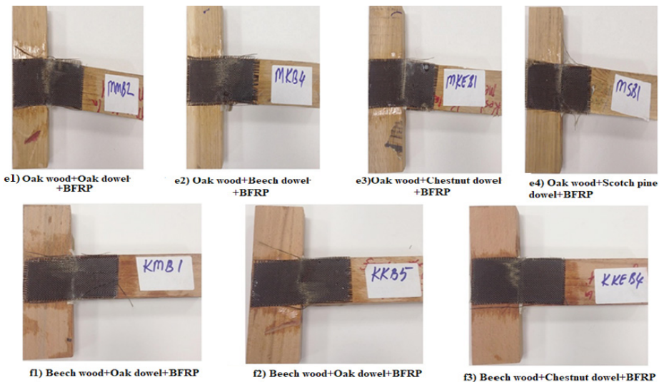
Figure 6: Mode of T-type, two pin dowel joint failure reinforced with BFRP.
