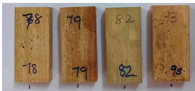
Figure 2: Rubberwood blocks after 2 years of exposure to L. africanus as per IS (4873 Part 2 2008).
