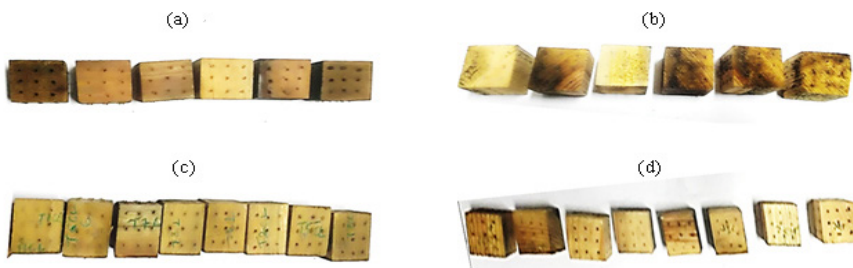
Figure 6: Treated and Control Blocks (a) Control TG, (b) Control SYP, (c) TG after T 3 , (d) SYP after T 3 ) (a) and (b) exhibits fungal growth whereas (c) and (d) remains unaffected.
