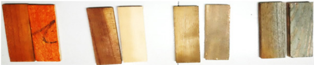
Figure 3: Veneer specimens exhibiting functional groups in treated and untreated samples (Red indicating Flavanoid, Green color indicating Phenol, Brown colour Alcaloid, Brown colour marking presence of terpenoid in treated and untreated veneers).
