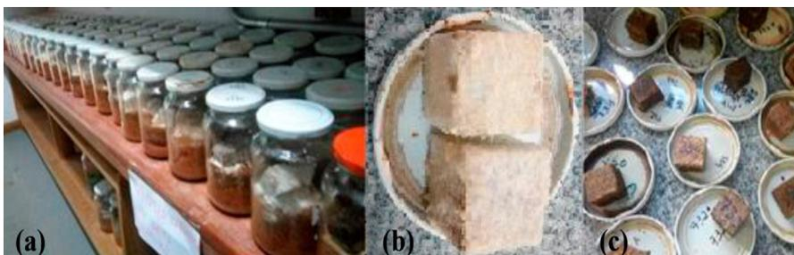
**Figure 2:** (a) Incubation room experiment; (b) Samples colonized by fungi; (c) Clean samples for oven drying.
