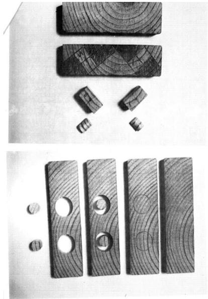
**Figure 3:** Examples of 12mm diameter plugs cut from the 127mm permeability specimen and used to determine longitudinal- (upper) and radial- (lower) gas permeability.
