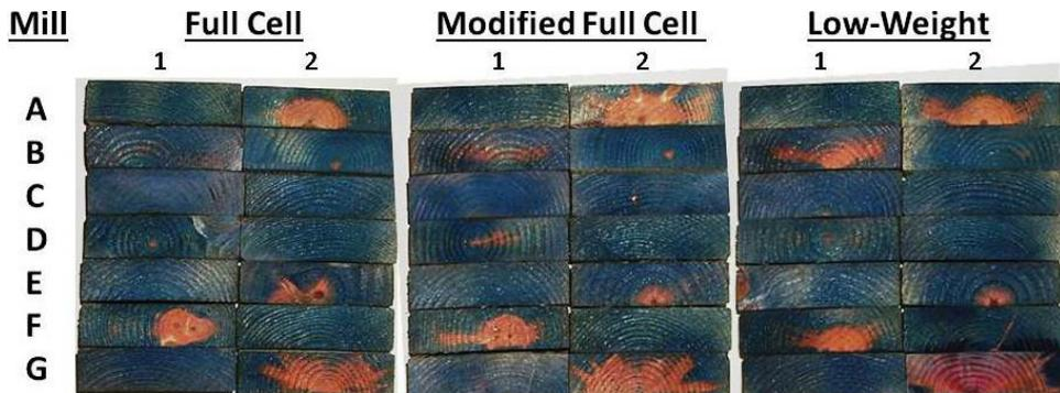
**Figure 4:** Matched treated lumber samples from Phase II showing CCA penetration patterns of two replicate 2x6 southern pine pieces from seven different Mills after either a full-cell, modified full-cell, or low-weight treatment. Locations of the seven mills sampled are given in Table 3.
