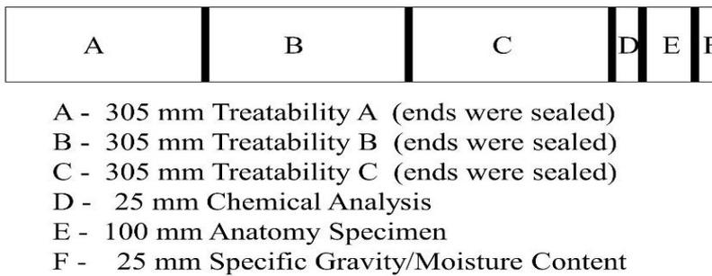
**Figure 2:** Example of Phase II cut-up pattern to obtain six samples from each of the 14 untreated 1,22 m long nominal 2x4 (38 x 89 mm) matched halves of Southern pine lumber.
