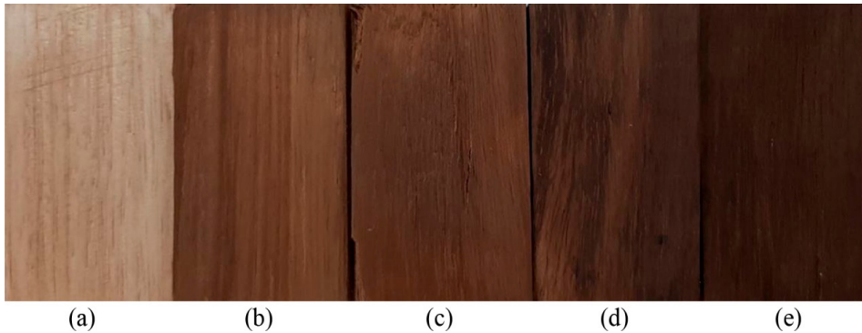
Figure 1: Color variation of the samples: (a) Untreated and heat-treated at (b) 155°C, (c) 165 °C, (d) 175°C, and (e) 185 °C.
