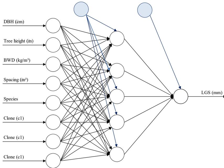
**Figure 1:** Artificial neural network structure model to estimate longitudinal growth strain with eight input neurons, five hidden neurons, and one output neuron.
