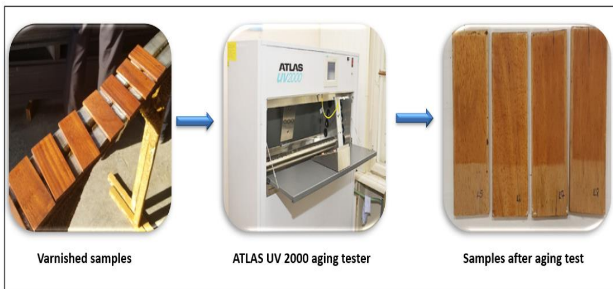
Figure 4: UV aging test application.
