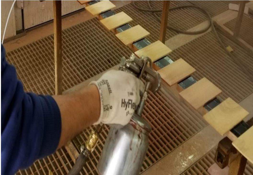
Figure 2: Varnishing application processes on wood samples.
