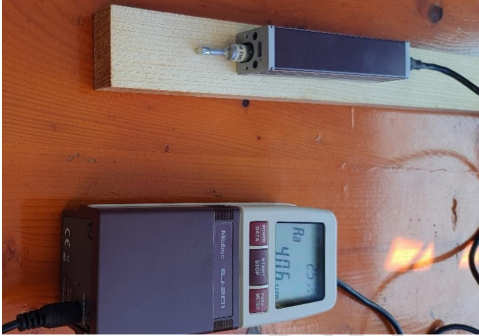
Figure 1: Measurement of radial section roughness in progress.
