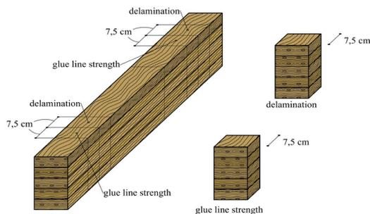
**Figure 4:** Removal specimens for delamination and shear strength tests on the glue line.
