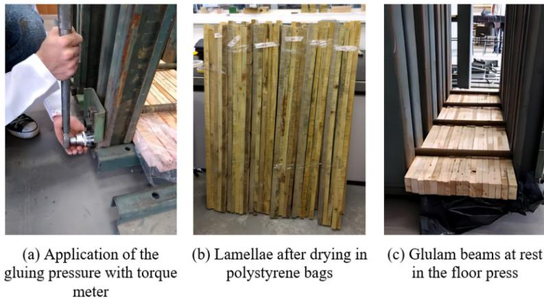
**Figure 3:** Fabrication of the Glulam beams.
