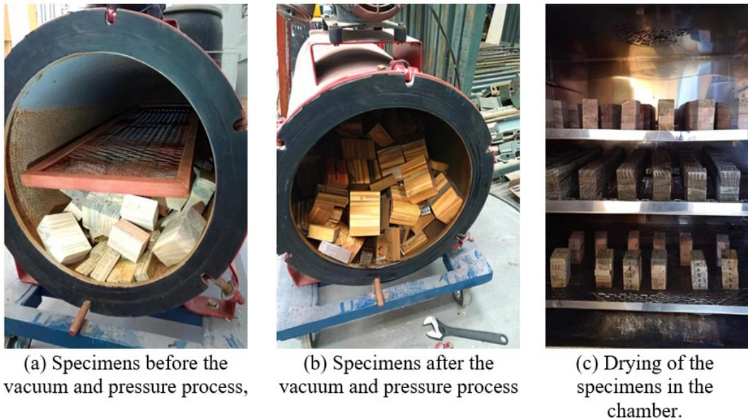
**Figure 5:** Details of the drying process.
