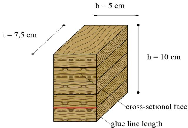
**Figure 6:** Cross-section considered in the delamination evaluation.
