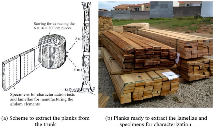
**Figure 1:** Slash pine (*Pinus elliottii* Engelm.) wood for manufacturing the Glulam elements.
