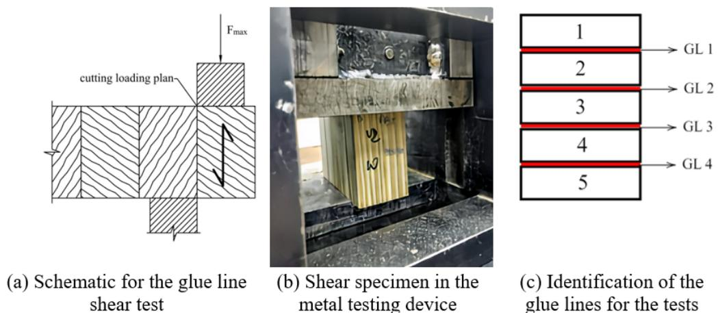
**Figure 7:** Details of the glue line shear test.
