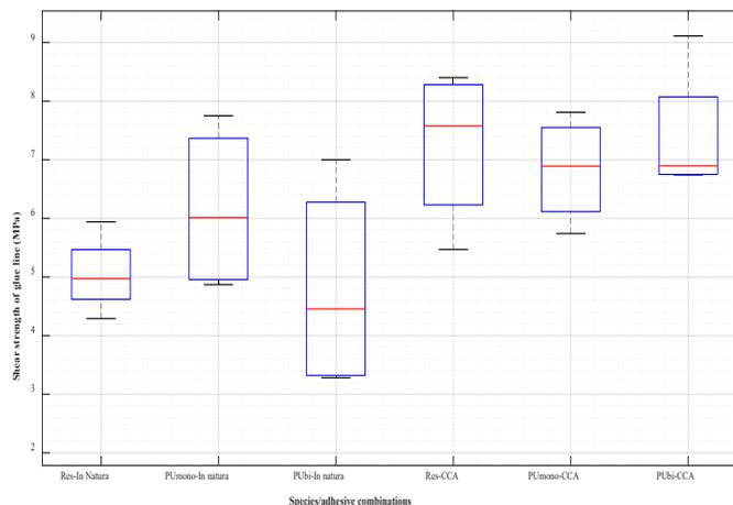
**Figure 8:** Boxplot for species/adhesive combinations considering the overall average of shear strengths obtained for all glue lines of the beams.
