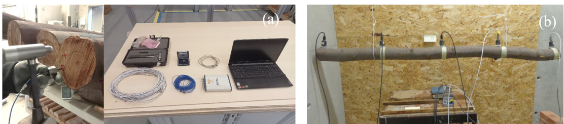
Figure 2: (a) Longitudinal Stress Wave and (b) Transverse Vibration testing.
