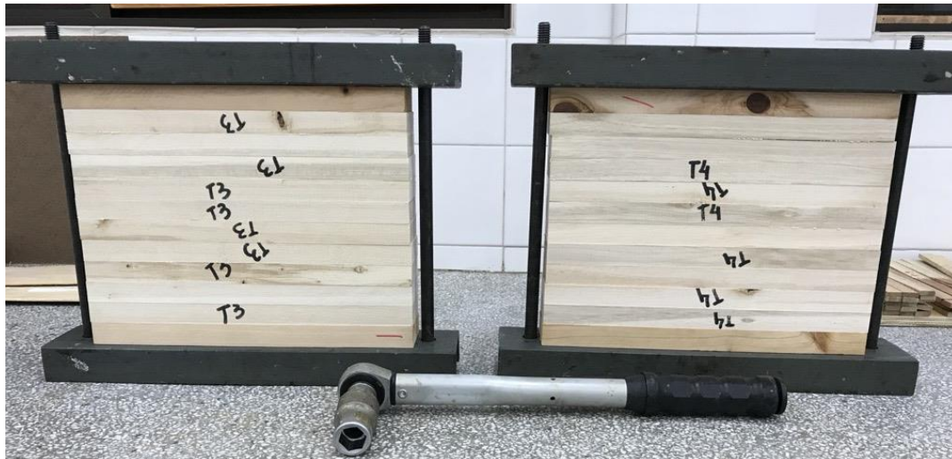
Figure 3: Joints glued and pressed.
