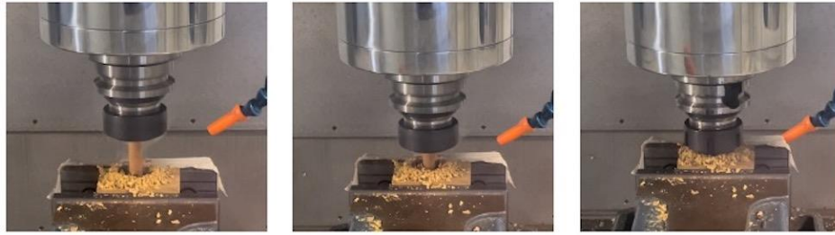
Figure 4: Dowel welding process.
