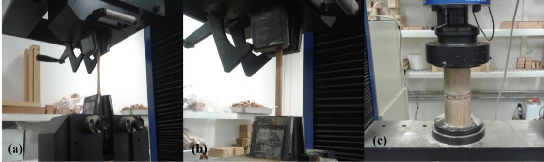
Figure 1: Mechanical tests performed on bamboo species. (a) Tensile strength parallel to grain, (b) Shear strength parallel to grain, (c) Compressive strength parallel to the grain.
