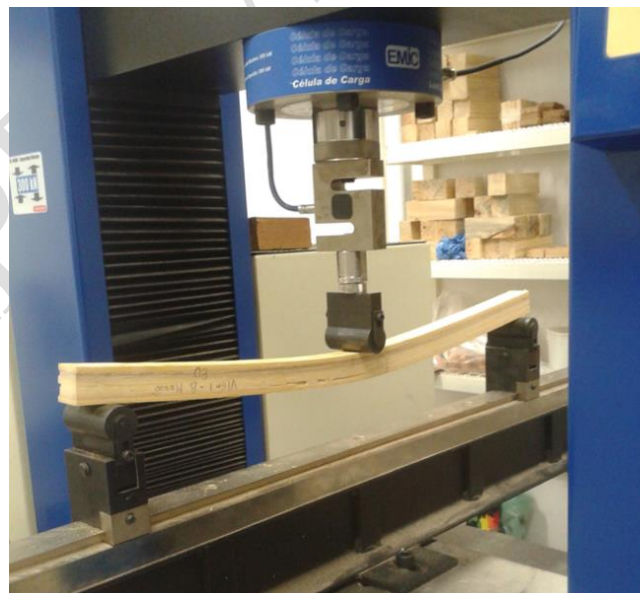
Figure 1: Three-point bending test performed on a LBL beam.
