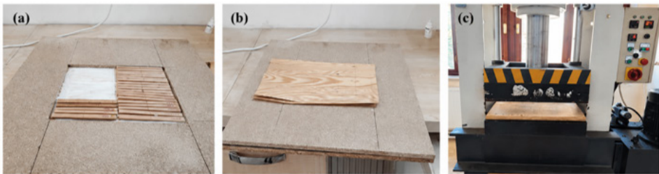
Figure 2: Lamination process. (a): Gluing the intermediate layers and placing them in the mold; (b): Placement of veneers; (c): Pressing process.
