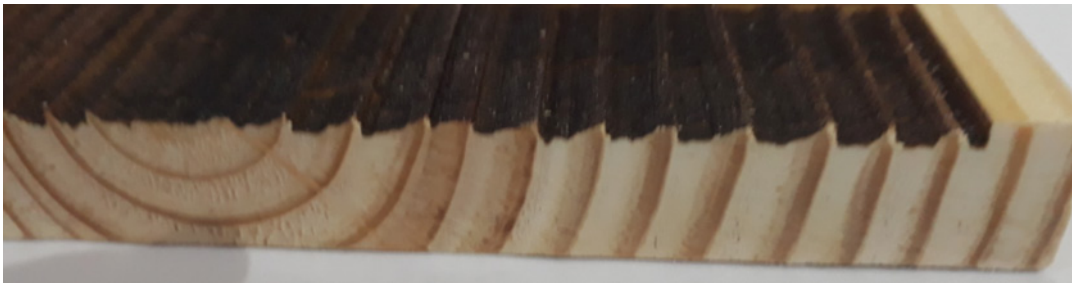
Figure 4: Laser engraving examples of anatomical structures of wood solid materials.
