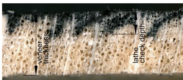
Figure 5: Cross-section with measuring parameters (lathe checks).
