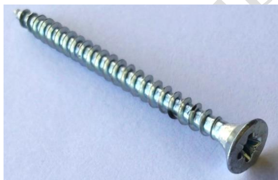
Figure 1: 4 x 50 mm screws used in the experiments.
