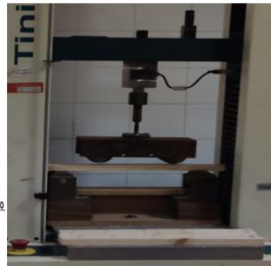
Figure 3: Setup and device of the four-point bending test.
