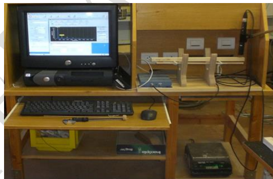
Figure 2: Device used for measuring the dynamic modulus of elasticity.
