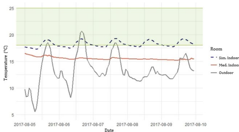
Figure 12. Outdoor and indoor temperatures in winter, simulated, without occupation, with improvements on the envelope. Source: Preparation by the authors in R.
