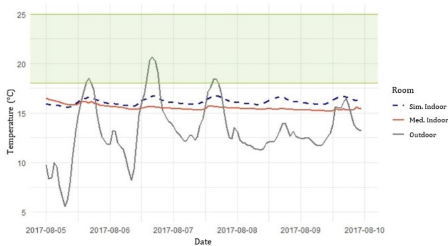
Figure 12. Outdoor and indoor temperatures in winter, simulated, without occupation, with improvements on the envelope. Source: Preparation by the authors in R.
