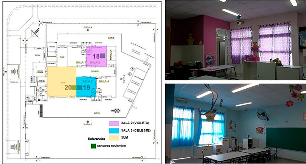
Figure 5. Left: JI 174 monitoring scheme. Period Nov. 12th, 2012 – Nov. 19th, 2012 Right.: Interior Room 2 (Violet), with NW-facing windows, and Room 3 (Light Blue), with SE-facing windows.
